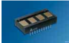
PD353X Display Parallel Input with a Character Set
