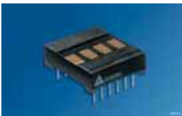
DLX1414 Display Parallel Input with a Character Set
