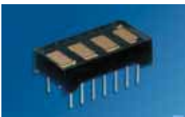
SLX2016 Display Parallel Input with a Character Set
